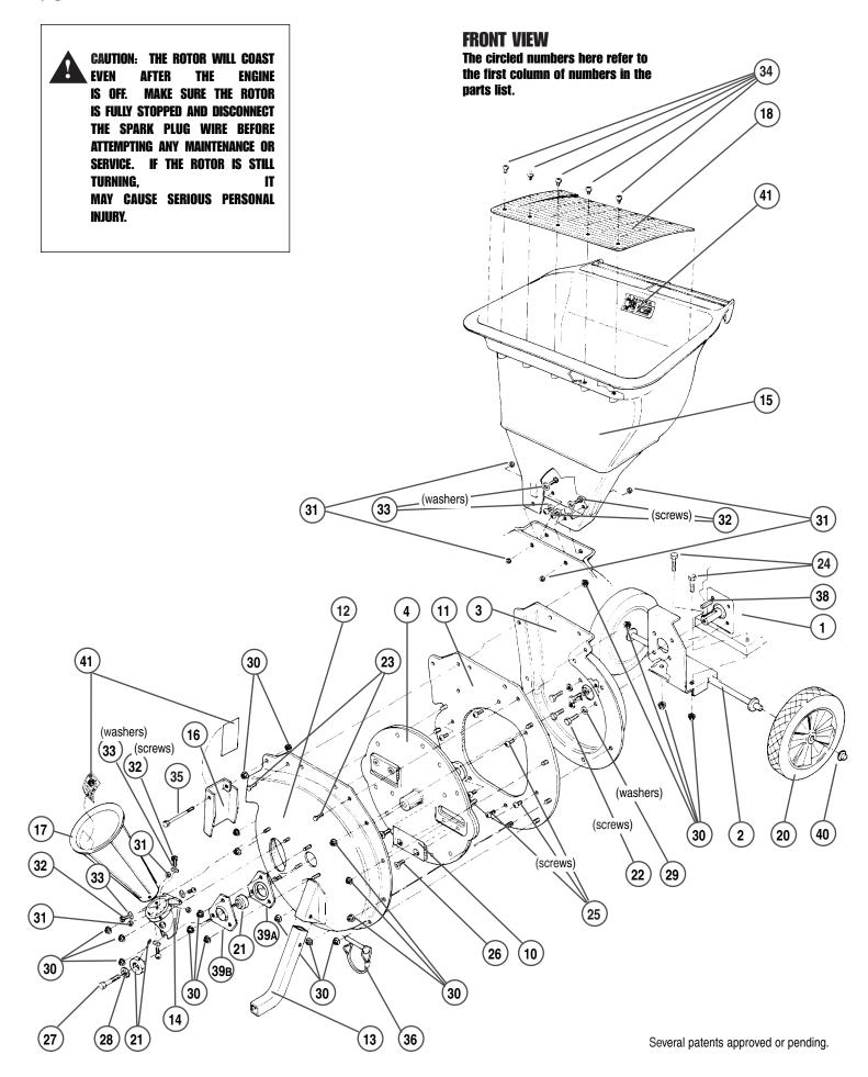
CAUTION: THE ROTOR WILL COAST EVEN AFTER THE ENGINE IS OFF. MAKE SURE THE ROTOR STOPS TURNING, THEN DISCONNECT THE PLUG WIRE FROM THE ENGINE BEFORE ATTEMPTING ANY MAINTENANCE OR CLEAN-OUT. IF THE R O T O R IS STILL TURNING, IT MAY CAUSE SERIOUS PERSONAL INJURY.
