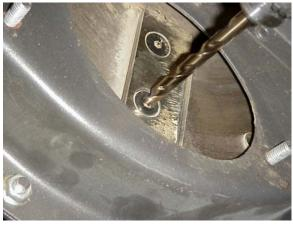
600 rpm and lubricate the hole frequently.
