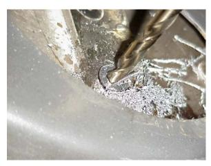
5. Stop drilling and remove the head from the drill bit.
