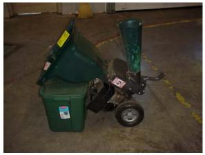
2. Remove chipper cone using ½" wrench and rotate rotor so that chipper knife is visible through opening. If necessary, remove the spark plug to make it easier to rotate the rotor.
