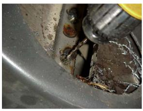
threads on the rotor. Drill completely through the screw shaft to allow proper insertion of the extractor.
