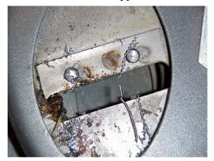
7. Place 7/64" drill bit in 3/8" variable speed drill. Again, the cobalt bit is recommended because the chipper knife screws are hardened and will ruin most bits. Do your best to drill down the centerline of the screw. For best results, run the drill slowly at 400 to 600 rpm lubricate and the hole frequently. The most important thing is not to damage the
